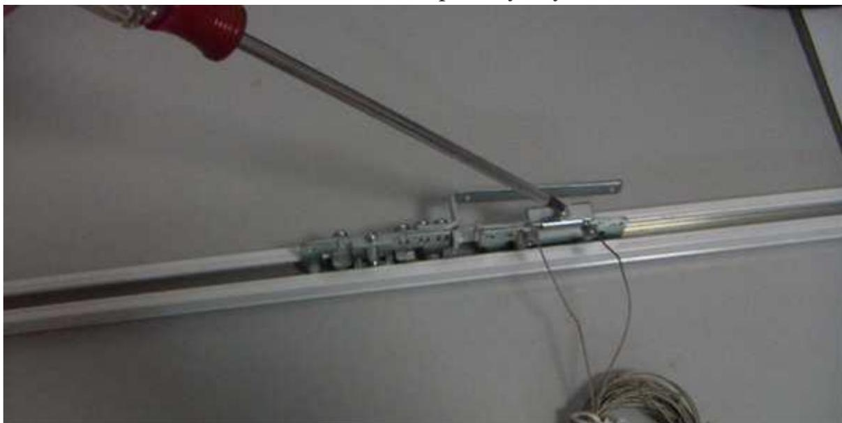
11. Slide the red-catch and insert the transmission box.
