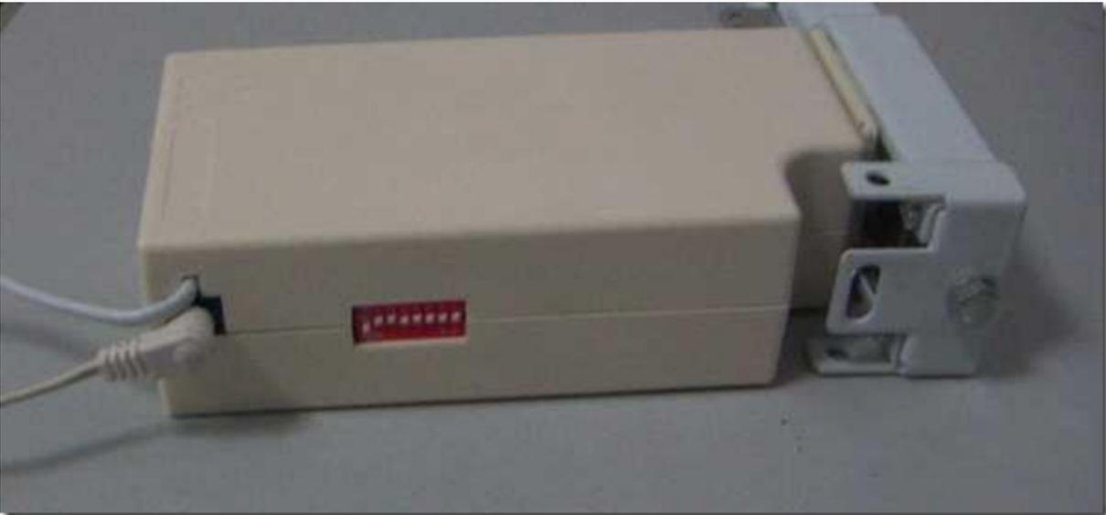
14. You are now able to perform the test-run without the curtains attached. The track should automatically stop when it is fully open or closed.
