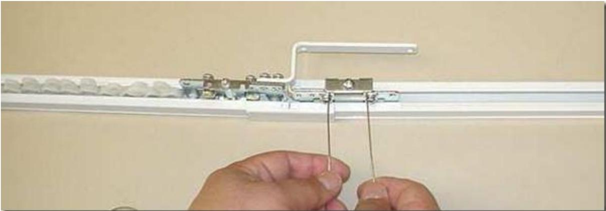
9. Loosen the hex bolt as much as possible with a spanner. This will be used to adjust the tightness of the steel wire in step 14 and keep the curtains from automatically closing when fully open or closed.
