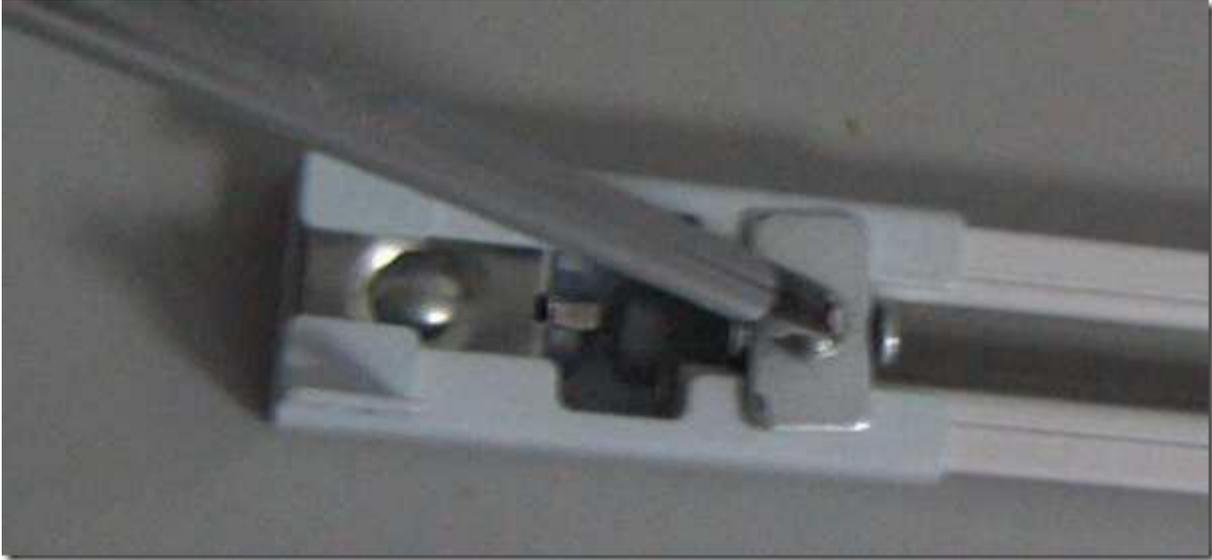
8. Pull the steel wire and make it even in both sides.
