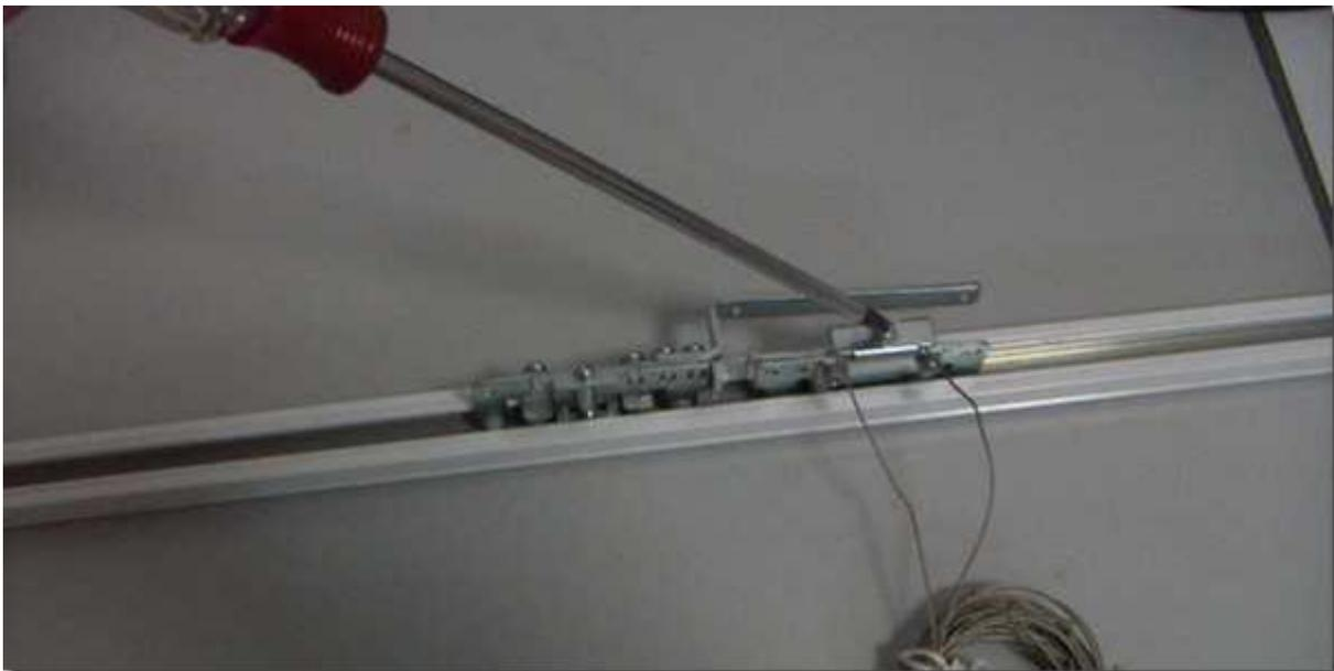
3. Remove the end-base screw for track extension.
